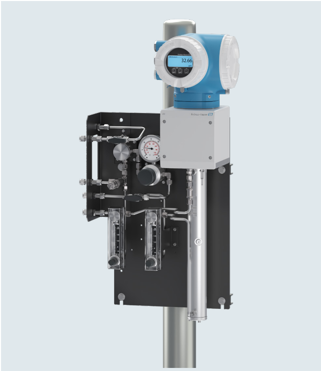
J22 on panel with sample conditioning system, pole mounted using pole mount kit
