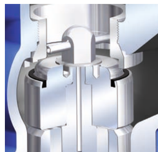
Permanent leak proof performance due to soft sealing plug (PREDEX® / PREDU®)
