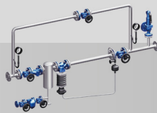
e.g. pressure reducing station PREsys®
