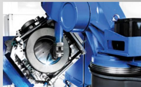
The sealing surface is coated with stellite by a fully automatic welding robot with an integrated measuring system. All CNC programs are developed by our expert in-house programmers. The precise synchronisation of the welding system's eight axes ensures high product quality.
