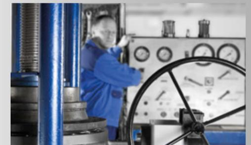
Every ZETRIX® process valve is leak-tested according to DIN EN 12266. The test pressures and times are stored on our computer aided test bench. Special tests can also be performed at the customer's request.
