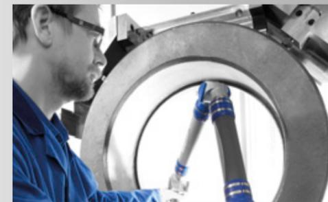
With the three-dimensional measuring system, the valves can be measured and scanned against 3D data and subsequently evaluated and saved on a PC. The measurements are carried out directly in the machine to ensure reliable production processes.
