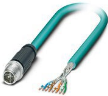
Figure 36 Network cable, Ethernet CAT6A (10 Gbps), CC-Link IE CAT6A (10 Gbps), 8-position halogen-free, shielded (Advanced Shielding Technology), Plug straight M12 / IP67, coding: X, on free cable end, coding: X
