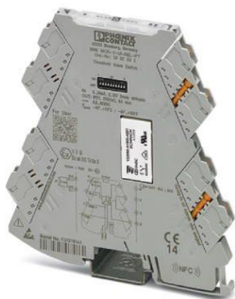
Figure 44 Limit value switch. Universally configurable limit value switch with PBT relay output and plug-in connection technology for switching analog limit values. Configurable via DIP switch or software. Push-in connection technology, standard configuration.
