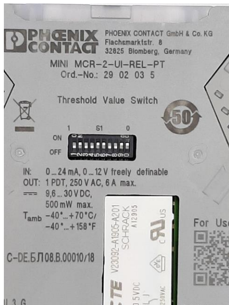
Figure 33 Physical DIP switch configuration for Low alarm functions. DIP switches 3, 5, 6, 9, 0 activated 'ON'
