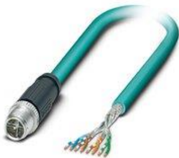
Figure 45 Network cable, Ethernet CAT6A (10 Gbps), CC-Link IE CAT6A (10 Gbps), 8-position halogen-free, shielded (Advanced Shielding Technology), Plug straight M12 / IP67, coding: X, on free cable end, coding: X
