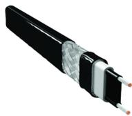
nVent RAYCHEM BTV self-regulating trace heating cables provide freeze protection and process temperature maintenance, up to 150 °F/65 °C, of pipes/vessels without steam cleaning requirements. They withstand intermittent exposure to 185 °F/85 °C and are hazardous area approved. The polyolefin outer jacket (-CR) is suitable for mild inorganic solutions. The fluoropolymer outer jacket (-CT) provides high chemical resistance against aggressive organics and corrosives.
