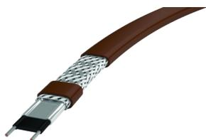
nVent RAYCHEM QTVR self-regulating trace heating cables are suitable for freeze protection of large pipes/vessels with high heat loss, and for process temperature maintenance applications without steam-cleaning requirements, up to 225 °F/110 °C. The fluoropolymer outer jacket (-CT) provides high chemical resistance against aggressive organics and corrosives.
