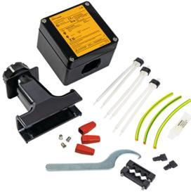
nVent RAYCHEM T-100 is a cold-applied high profile splice or tee connection kit for trace heating cables in both non-hazardous and hazardous locations. Mounted on the pipe, through the thermal insulation and cladding. Includes cold-applied heating cable core sealer.
