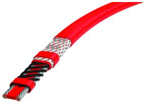
nVent RAYCHEM XTV self-regulating trace heating cables are mainly used for freeze protection of pipes and vessels that require steam cleaning and process temperature maintenance, up to 250 °F/121 °C. They withstand intermittent exposure to 482 °F/250 °C. The fluoropolymer outer jacket (-CT) provides high chemical resistance against aggressive organics and corrosives.
