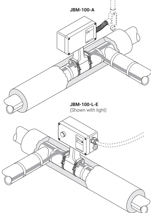
The Raychem JBM-100 kit serves as a power connection, splice, or tee for up to three Raychem brand BTV, QTVR, XTVR, HTV or VPL heating cables. It is approved by FM, CSA, PTB and IEx for use in hazardous locations.
