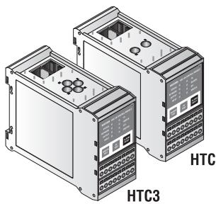
Two versions of this module are available: The NGC-40 Control module for single-phase heaters, NGC-40-HTC; the NGC-40 Control module for three-phase heaters, NGC-40-HTC3. Both versions use temperature data to control one single heat-tracing circuit by switching of Electromechanical relays (EMR) or Solid-State Relays (SSR). The NGC-40-HTC/HTC3 also provides ground-fault (leakage) current and line current sensing, monitoring and alarming.
