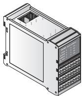
Each Input Output Module, NGC-40-I0, installed in the panel provides up to four (4) additional RTD inputs. These additional RTD inputs can be assigned to any NGC-40-HTC/HTC3 module. The NGC-40-I0 module also provides one alarm relay that can be connected to an external annunciator and one digital input that is programmable and may be assigned to any NGC-40-HTC/HTC3 module for various functions such as forcing the contactor or SSR on or off.
