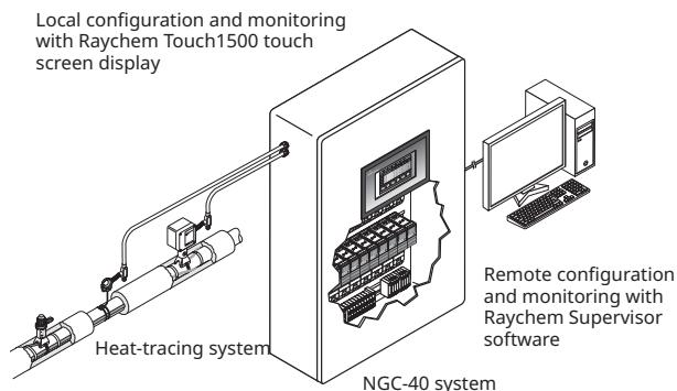
The Raychem NGC-40 is a multipoint electronic control, monitoring and power distribution system with a unique single-point controller architecture for heat-tracing used in process temperature maintenance and freeze protection applications. By taking advantage of innovative modular packaging techniques, the Raychem NGC-40 system provides configuration and component flexibility so that it may be optimized for a customer's specific needs.
