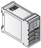
The NGC-40-BRIDGE module provides the interface between a panel's internal CAN-based network and upstream devices. Multiple communication ports are supported, allowing serial and Ethernet connections to be used with external devices: Each Bridge Module has two RS-485 ports, one RS-232 port and one 10/100Base-T Ethernet network with programmable communication parameters. A maximum of 80 NGC-40 modules, a combination of HTC, HTC3 or I/O modules, can be connected to one NGC-40-BRIDGE module.
