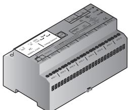
A Remote Monitoring Module (RMM2) is used to collect temperatures for control and monitoring of the heat-tracing system by the Raychem NGC-40 control panel. The RMM2 accepts up to 8 RTDs that measure pipe, vessel, or ambient temperatures. A single twisted-pair RS-485 cable connects up to 16 RMM2's for a total monitoring capability of 128 temperatures. The RMM2's are placed near desired measurement locations in nonhazardous or hazardous locations.
