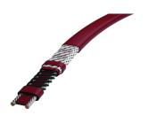
nVent RAYCHEM KTV self-regulating trace heating cables are mainly used for process temperature maintenance of pipes/vessels that require steam cleaning, up to 300 °F/150 °C. Also used for freeze protection of systems with high heat losses. They withstand intermittent exposure to 482 °F/250 °C. The fluoropolymer outer jacket (-CT) provides high chemical resistance against aggressive organics and corrosives.
